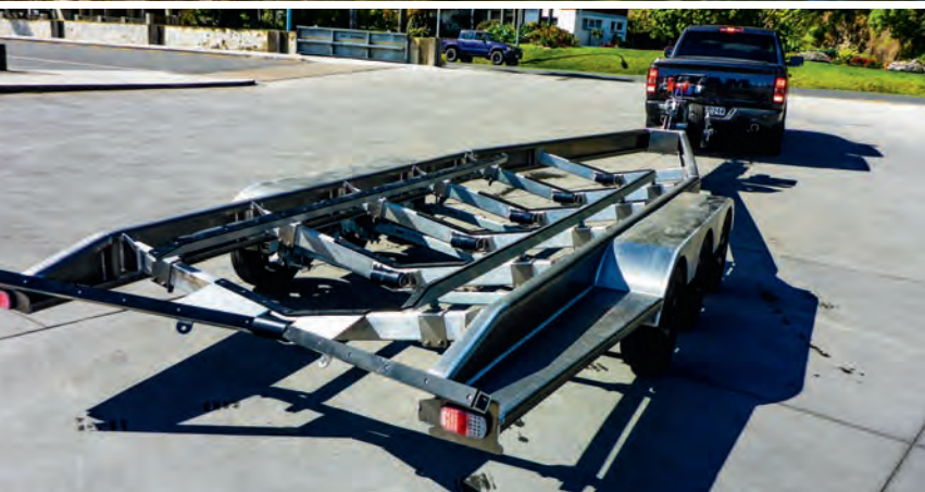
GFAB built the alloy trailer. It's designed for drive-on, drive-off retrieving and launching with keel rollers, bunk and skids.
