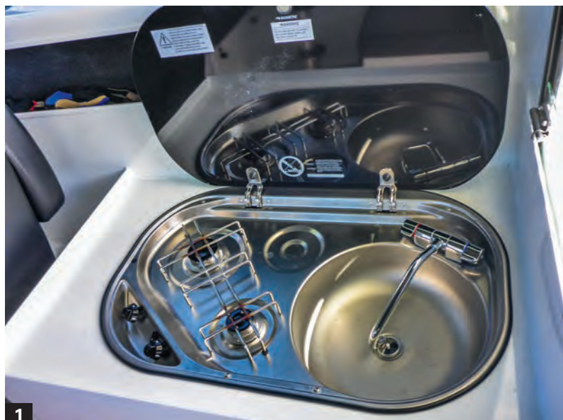
1) The galley includes a two-burner hob and freshwater system. 2) Two rear windows recess into the bulkhead; rear-facing bench seats are ideal for watching lures. 3) A pull out hot and cold freshwater shower is fitted in the cockpit.
