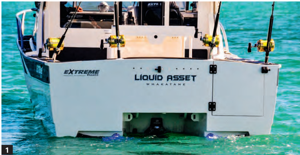
1) The leg is set into a bay under the transom and allows walk-around space behind the engine; 2) Liquid Asset is powered by a six-cylinder Mercury QSD 4.2 litre, 320hp diesel inboard; 3) The rig produced a remarkable 8.9 knots in reverse! Opposite page: The boat rode softly and could turn on a dime without any concern.
