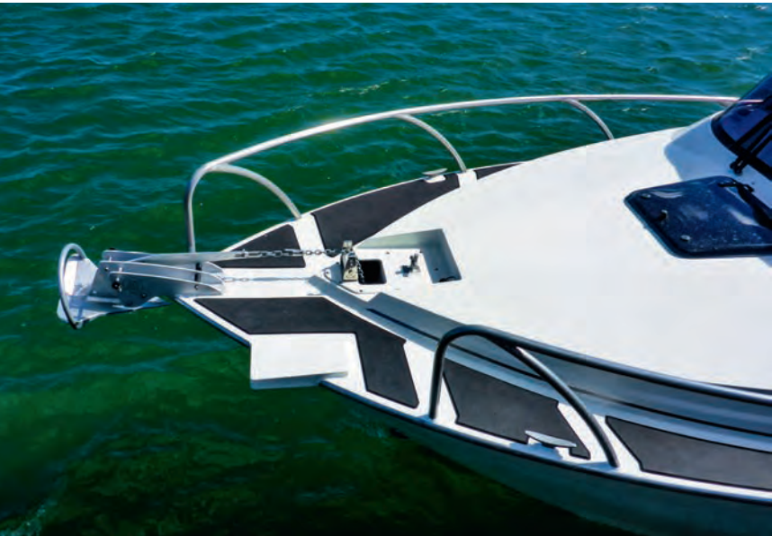
Towards the bow, the rails are dissimilar to allow for an electric outboard mount.
